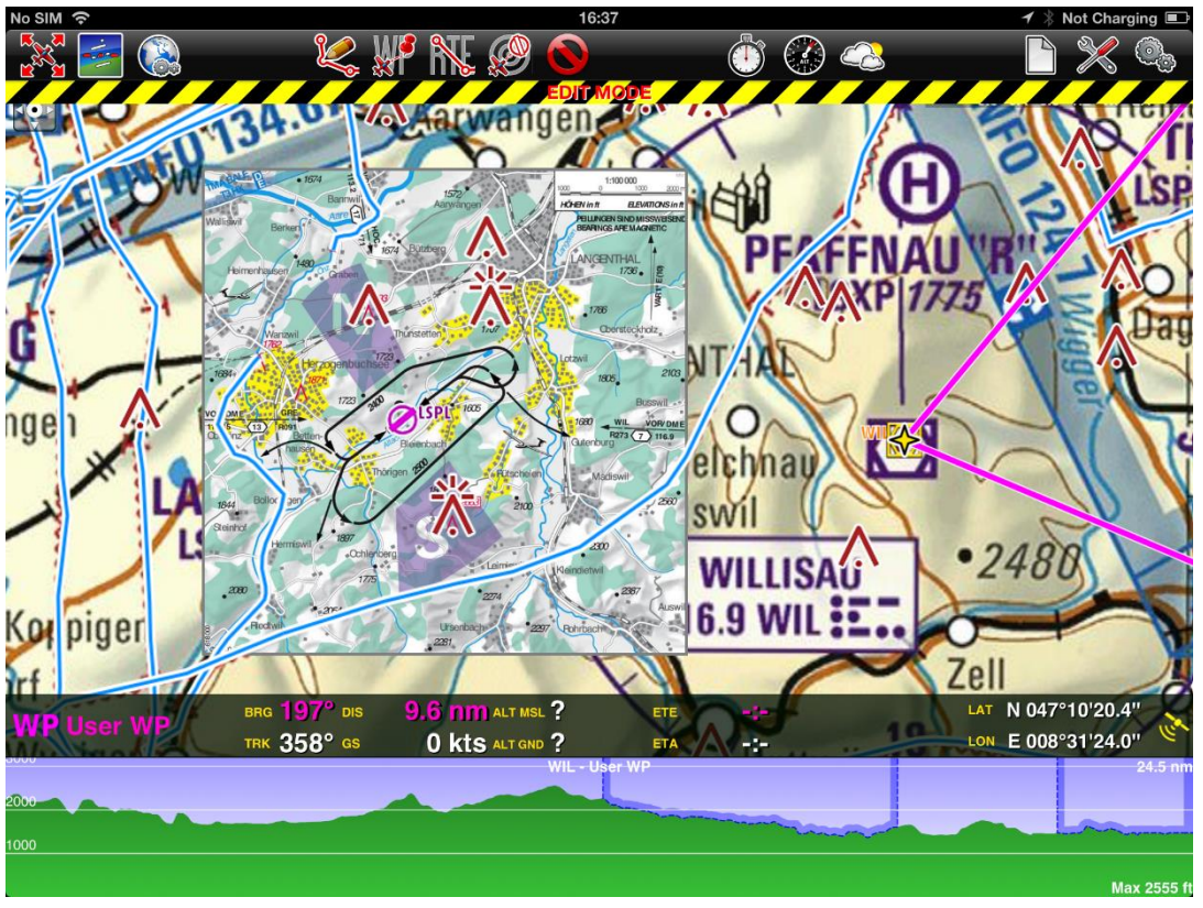
Either automatic or “enforced” displaying of approach charts (referenced) on moving map:
